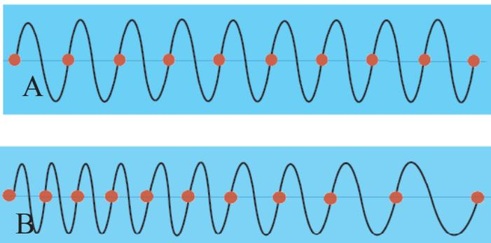
Figure G-4. These sine waves represent signals generated by a Cesium clock. We use them to measure the size of the time unit. In graph A there is no change in the size of the time unit as indicated by the equal distance between the red dots. In graph B the size of the time unit is increasing as one moves to the right.
